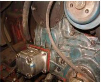
(f) Installation of the pump command
