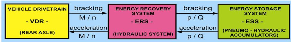
Fig. 3. Global systemic model of a motor vehicle equipped with a kinetic energy recovery system.
