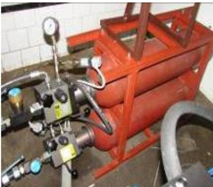
e) The accumulating subsystem
