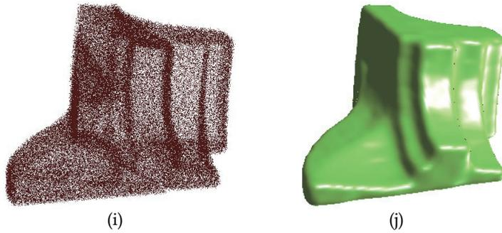
Fig. 10. Examples of fan disk. (a) Sparse point clouds. (b) Resulting surface of sparse point clouds. (c) Noisy point clouds. (d) Resulting surface of noisy point clouds. (e) Point clouds with holes and details. (f) Resulting surface of (e) and details. (g) Point clouds containing overlapping regions and details. (h) Resulting surface of (g) and details. (i) Hybrid defective samples. (j) Resulting surface of Hybrid defective samples.
